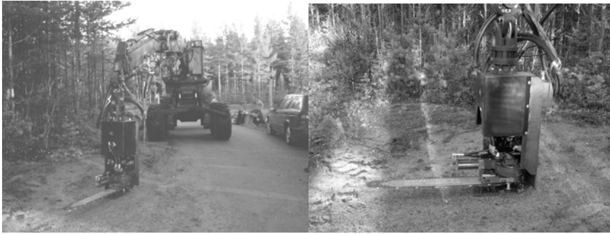
Figure 3. The base machine and prototype felling head used in the experiments.
