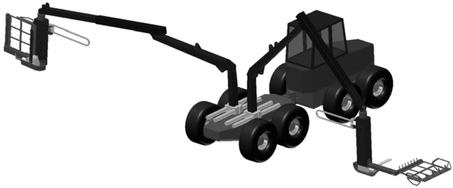
Figure 16. Hypothetical harvester with two cranes for simultaneously felling and bunching in boom-corridors. Sketch by Hans Nilsson (Robotcentrum Norr AB, Umeå, Sweden).
