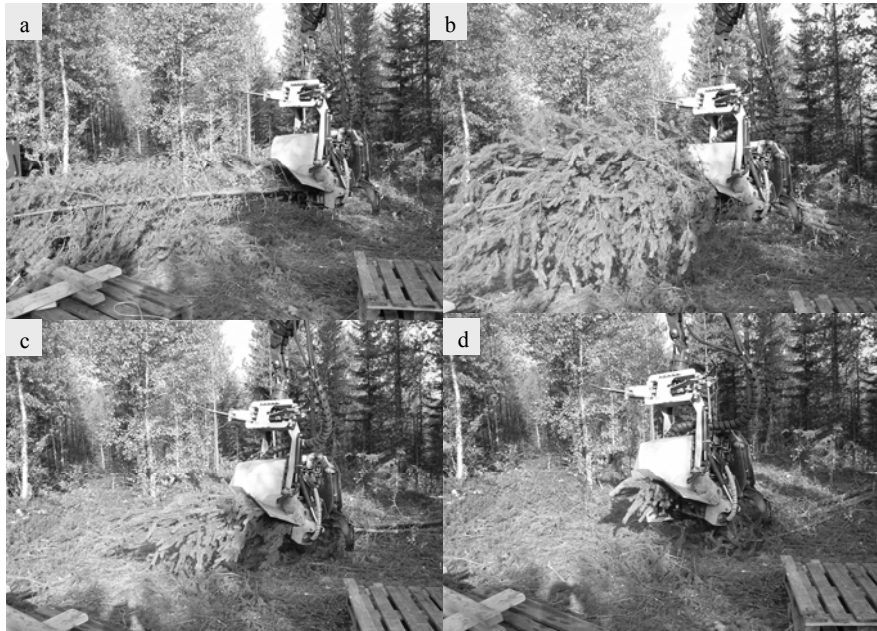
Figure 7. The compression and semi-debranching sequence of a bunch processed from the butt end (a) to the top end (d).
